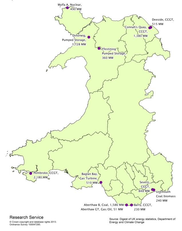
Notes: CCGT stands for Combined Cycle Gas Turbine. Pumped storage systems are a type of hydro-electric power generators which utilise off-peak electricity from the National Grid to elevate water. During periods of peak demand the water is released to generate electricity. These stations are net consumers of electricity and do not contribute to the generating totals analysed in this paper.
